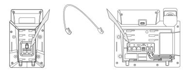
If you connect two expansion modules, connect the Ext out jack of the previous expansion module and the Ext in jack of the second expansion module using another supplied cord.
