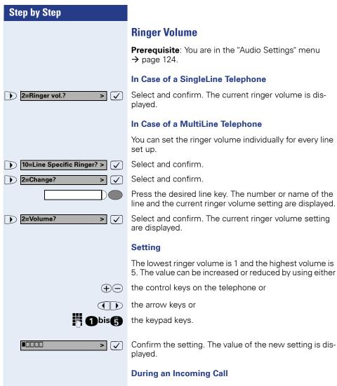
When your telephone rings at an incoming call, you can vary the volume of the ringer tone by means of the keys  $\oplus$  and  $\bigcirc$ . Then press the  $\checkmark$  key to save the setting. Otherwise the setting will only apply to the current telephone call.
