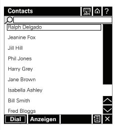
Find and select the relevant party in the list and then press the display key **Dial**. The phone number is used for this procedure.
