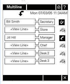
The sample displays on  $\rightarrow$  page 194 are standard Call Controls for an existing connection. However, the line information boxes can appear in all call views and all scenarios in which the line overview can be called up. They do not appear in a Call Control in which a caller can be put on consultation hold ( $\rightarrow$  page 157) or two calls are handled ( $\rightarrow$  page 162).
