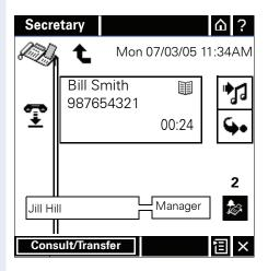
In the above example, two lines are ringing (including the one currently displayed); lines with lower priority status are only displayed if the calls are answered (by another telephone) or cleared down.
