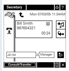
Consequently, the line informatiton box has the same function as the line control keys in the line overview. In this example, an incoming call is ringing on a **Manager** line.
