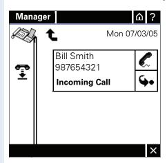
If a call is coming in on the prime line, the display switches immediately to Call Control without you having to press the **View Line Box** beforehand.
