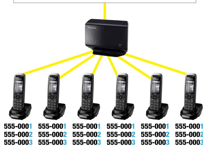
6 Station: 3 Line "Key" System
